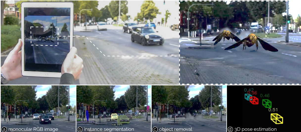
Figure 1: TransforMR is a video see-through mixed reality system for handheld devices that performs 3D pose-aware object substitution to create meaningful mixed reality scenes, enabling applications such as alternate mixed realities or real-time virtual character animation in context. (a) From just the monocular color camera of a mobile device, (b) TransforMR performs instance segmentation, (c) object removal, and (d) 3D pose estimation to substitute objects with pose awareness (top right).
