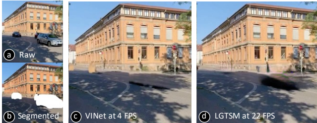
Figure 6: Exemplaric comparison of the two alternative real-time video inpainting methods, integrated in TransforMR. (a) Based on the monocular RGB frame, (b) TransforMR runs 2D instance segmentation to produce the inpainting bitmap. (c) With our adaptations in VINet, inpainting can operate at approximately 4 FPS without lag at a single VINet model instance and approximately 7 FPS with two load-balanced VINet model instances. VINet yields visually coherent inpainting for large masks. (d) With our adaptations in LGTSM, a chunk size of 4 frames, and downsampling to a width and height of 200 px, can operate at approximately 22 FPS, however at the cost of visual coherence for larger holes.
