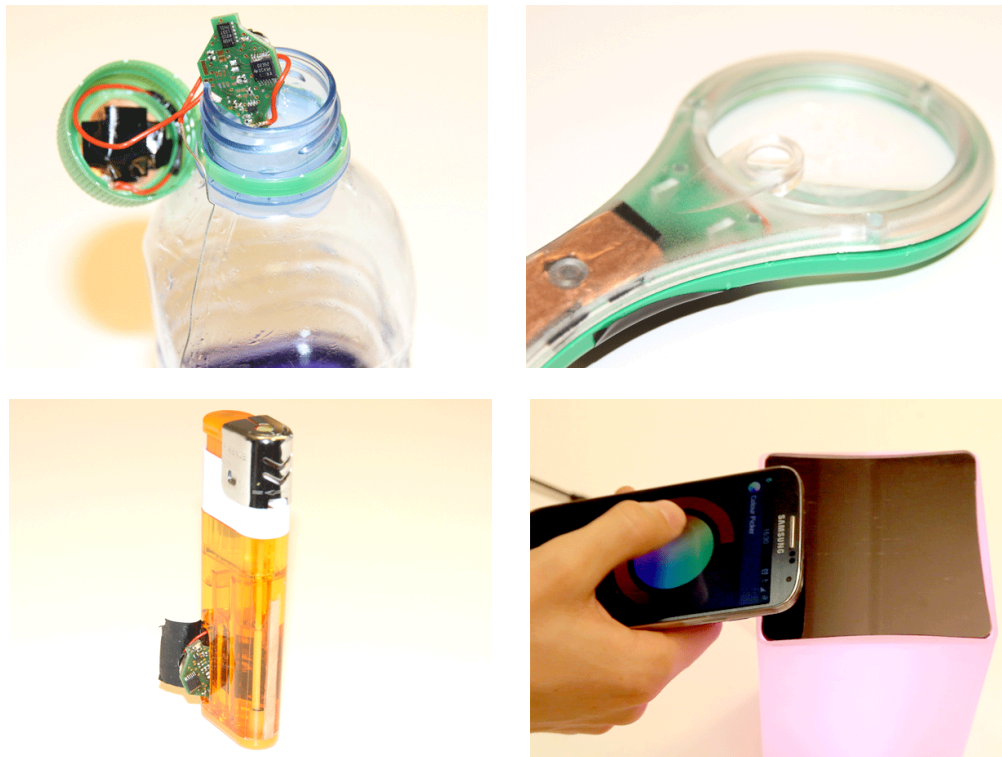
Figure 4.7.: Different electrode placements: (1) The transmitter electrode is placed directly under the bottle cap, (2) the magnifying glass has a big ground electrode in the region where the user touches the object, the transmitter electrode is placed around the glass, (3) the lighter uses its conductive part as a transmitter electrode, and (4) the mobile phone's transmitter electrode is placed at its back, the lamp's receiver electrode is under the black surface.
