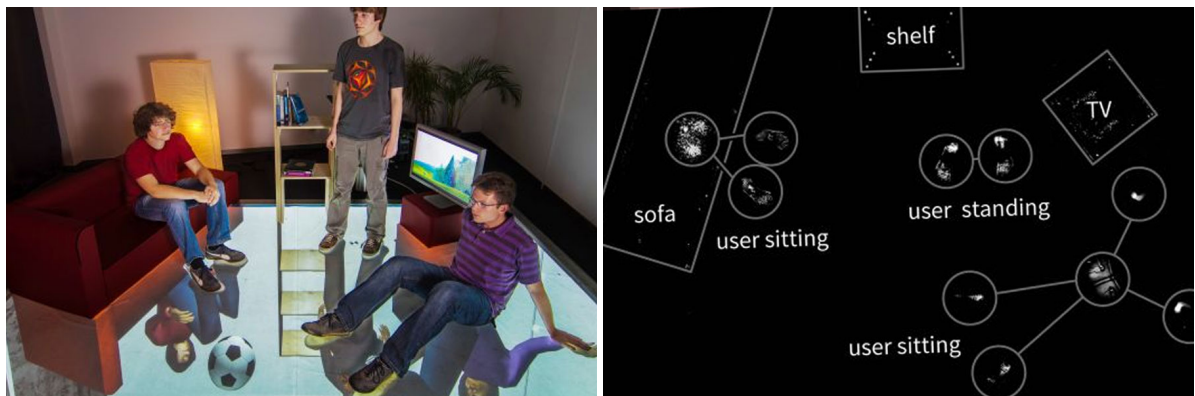
Figure 2.19.: Using large scale surfaces that generate reflections when being touched enable Braentzel et al. to derive body postures and identify users [BHH*13]. [BHH*13] © 2013 Association for Computing Machinery, Inc. Reprinted by permission.
