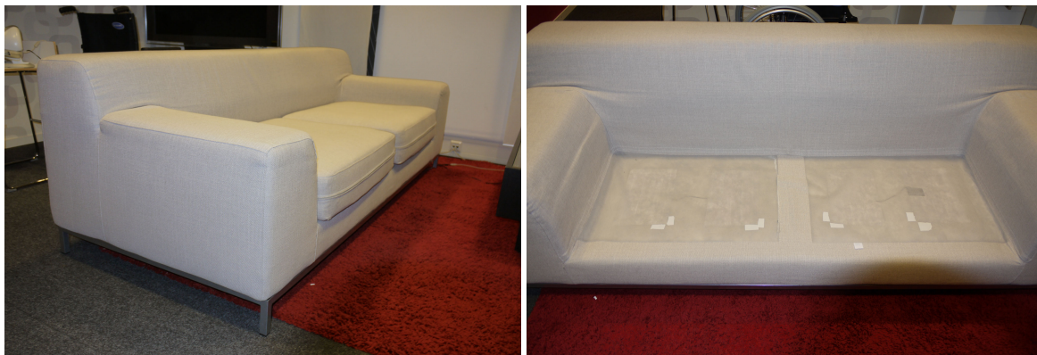
Figure 6.17.: An ordinary couch has been equipped with capacitive proximity sensors that have been set up under the upholstery and wooden elements
