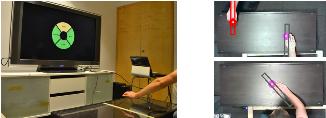
Figure 3.15.: CapTap controlling a multimedia application with radial menus. It is based on an array of OpenCapSense boards and an accelerometer to detect knocking and tapping [BZWK*14].
