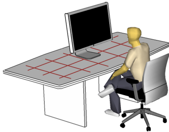
Figure 6.21.: The smart desk is equipped with a 3 by 5 grid of capacitive proximity sensors. The sensors measure the proximity to a user's body parts, for example the knees placed below the table, or the hands placed upon the table.
