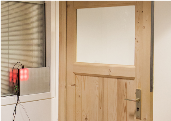
Figure 7.9.: The minimalistic feedback shows the state of the door - which is currently locked (red).
