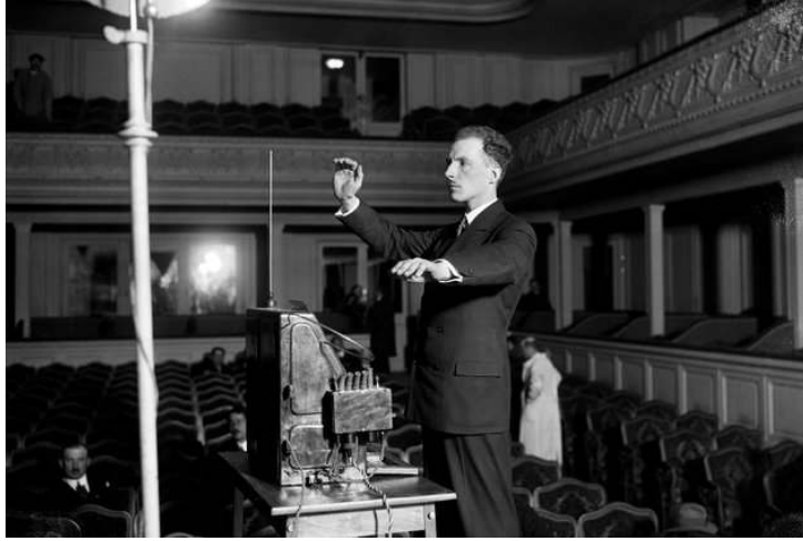
Figure 2.2.: Leon Theremin playing his music instrument based on capacitive sensing. The instrument adjusts its volume and frequency based on the proximity to body parts.
