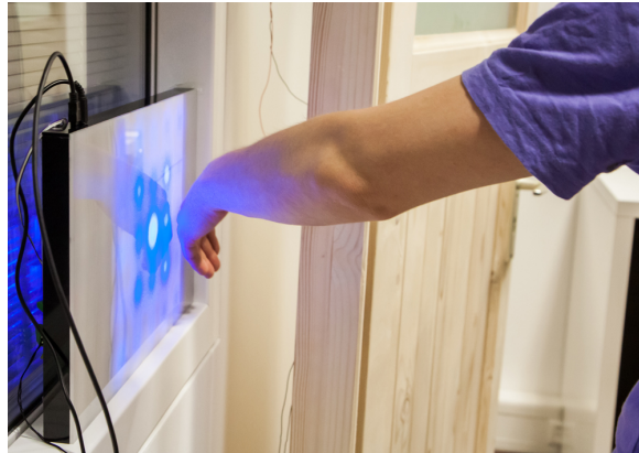
Figure 7.10.: The extended feedback also indicates when a hand approaches the gesture-recognizing surface.
