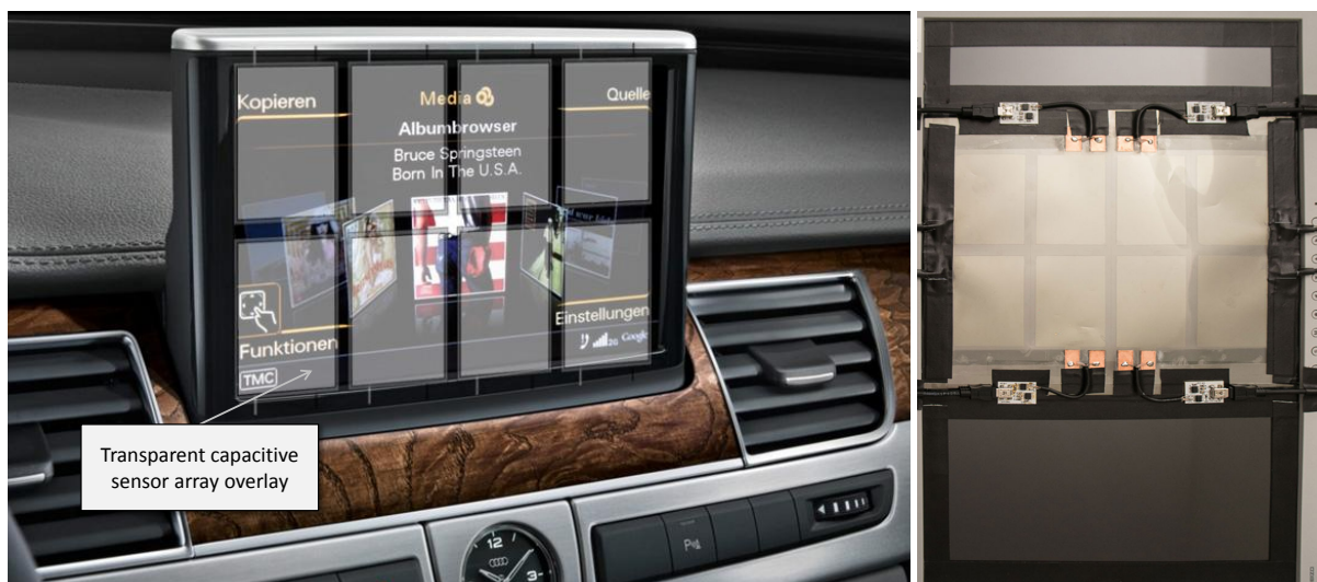
Figure 5.16.: The GestDisp prototype allows for interacting in front of a screen in distances up to 10 cm [Ber12]. On the right, an envisioned usage scenario in a car is depicted, the actual prototype is shown on the left.
