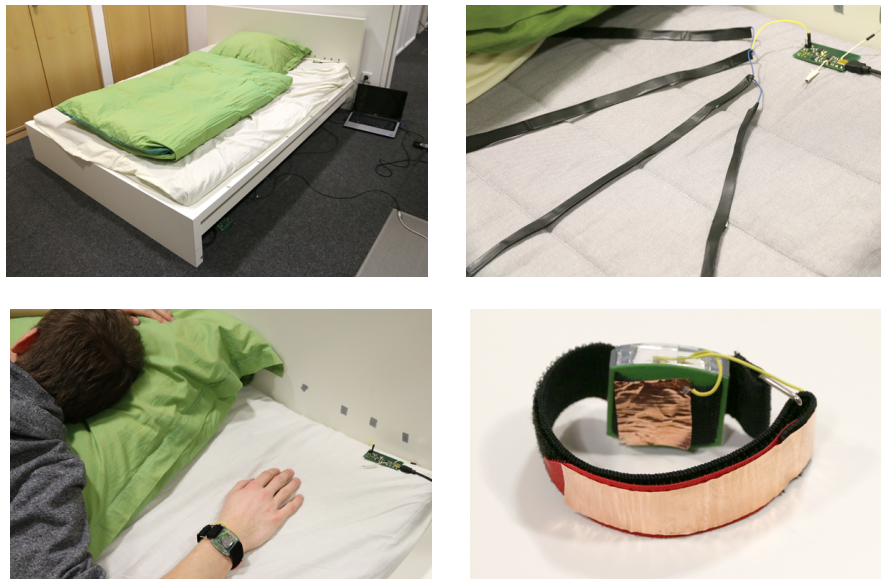
Figure 4.20.: A bed that is able to receive messages from multiple body-worn sensors, for example a wrist-worn accelerometer. The accelerometer is grounded using ground-coupling by touch (inner electrode) and transmits its sensor values to the bed (outer electrode).
