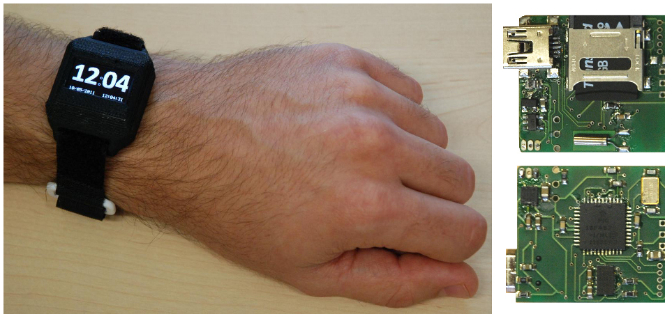
Figure 6.3.: The inertial data logger featuring a low-power microcontroller, a 3 axis accelerometer, a microSD flash card for storing the sensor data and a USB connector for accessing the data (on the right) is powered by a small lithium polymer battery and is packaged into a plastic case to be worn at the wrist (a version with an OLED display).
