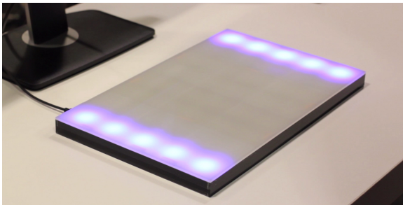
Figure 7.7.: Interactive regions are visualized with a glow effect. When the hand moves over the corresponding region, an application-specific action is triggered (e.g. scrolling).
