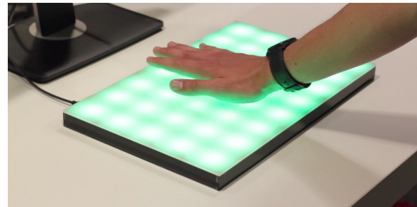
Figure 7.8.: When a gesture is recognized successfully, the device lights up in green. Moreover, it is possible to indicate unrecognized or unsupported gestures by lighting up in red.
