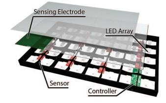
**Figure 2:** The gesture recognition device consists of four main components depicted in the figure.
